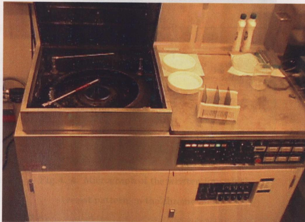
Fig.4.3 Automated developing machine
