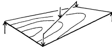
Fig. 2. Plate shear test for full-size plywood.
