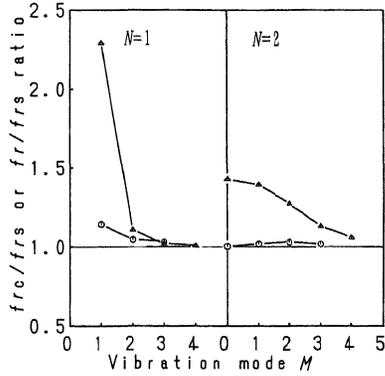
Fig. 8. Relationship between  $f_{r_c}$ -to- $f_{r_s}$  or  $f_r$ -to- $f_{r_s}$  ratio and vibration mode (M, N).
