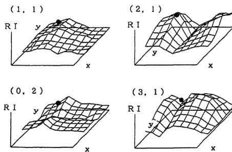
Fig. 5. Effect of tap position on relative spectrum intensity RI of some vibration modes.
