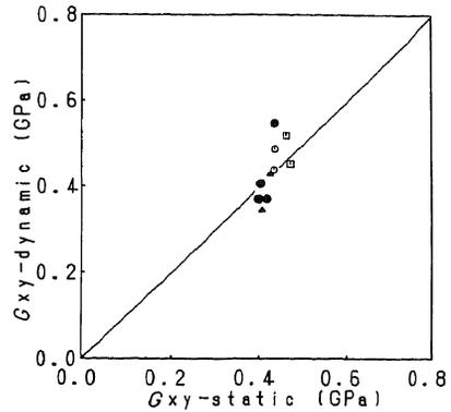
Fig. 9. Relationship between static shear moduli of small specimens,  $G_{xy}$ -static, and dynamic shear moduli calculated from resonance frequencies of higher-ordered vibration modes of full-size plywoods,  $G_{xy}$ -dynamic.
