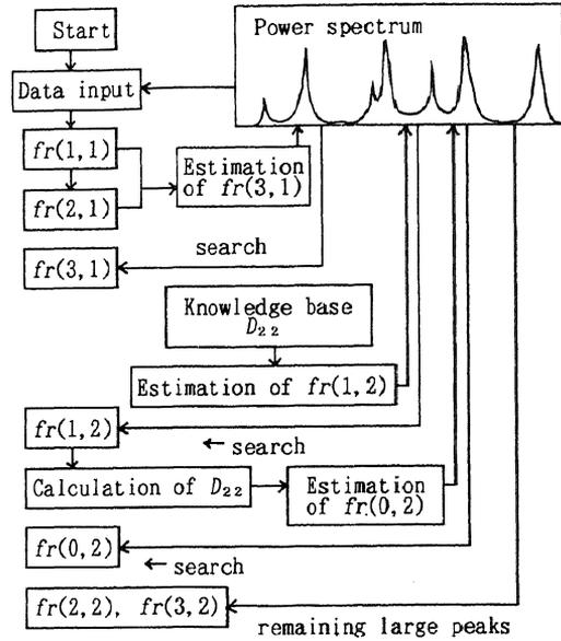
Fig. 4. Flow-chart of computer identification of spectrum peaks.
