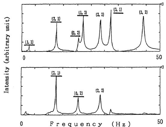
Fig. 6. Typical power spectra of full-size plywood.
