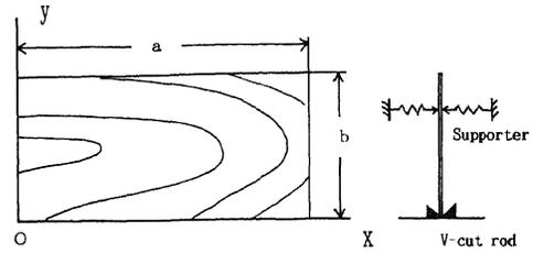
Fig. 1. Specimen support and coordinate system.
