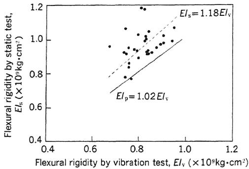
Fig. 2. Prediction formula of  $EI$  from vibration tests.
