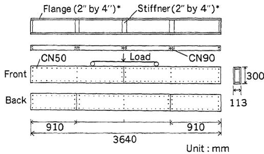
Fig. 1. Construction of plywood-webbed box beams.
