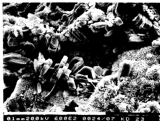
Fig. 2 Subequal amounts of clinoptilolite and smectite lining framework clasts in a porous sandstone. Hair-like fibres are mordenite. Authigenic growth of these minerals is considered to be contemporaneous. (Sample AU 42032)
