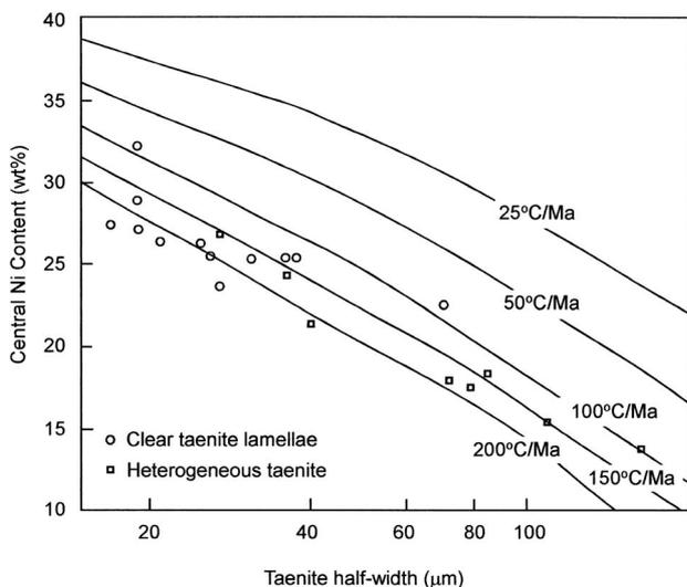
Fig. 8 Cooling rate curves for Toluca meteorite (Saikumar & Goldstein, 1988). Central Ni contents and half-width of clear and heterogeneous taenite in Toluca meteorite fall between calculated  $100 \sim 200^\circ\text{C}/\text{Ma}$  cooling rate curves.
