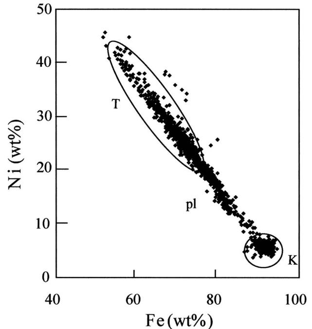
Fig. 5 Fe versus Ni contents for Fe-Ni alloy in Toluca iron. Fe-Ni alloy are composed of K, kamacite; T, taenite; and pl, plessite, which is the intergrowth or interface of kamacite and taenite.
