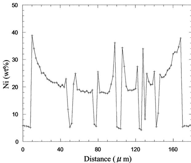
Fig. 7 Ni profile across the kamacite - heterogeneous taenite having plessite texture - kamacite in the Toluca meteorite.
