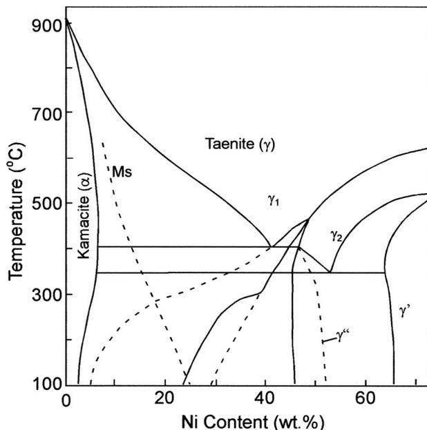
Fig. 1 Fe-Ni phase diagram determined by investigation of meteoritic metal. On this diagram,  $\alpha$  represents a low-Ni kamacite,  $\gamma$  represents a high-Ni taenite phase,  $\gamma^1$  represents a low-Ni paramagnetic bcc phase,  $\gamma^2$  represents a high-Ni ferromagnetic fcc phase,  $\gamma^3$  represents ordered  $\text{Ni}_3\text{Fe}$ ,  $\gamma^4$  represents ordered FeNi, and Ms represents martensitic transformation starting temperature (Yang *et al.*, 1997).
