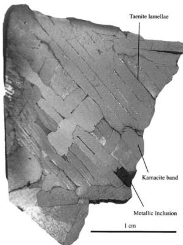
Fig. 3 Widmanstätten structure in the coarse octahedrite, Toluca meteorite.
