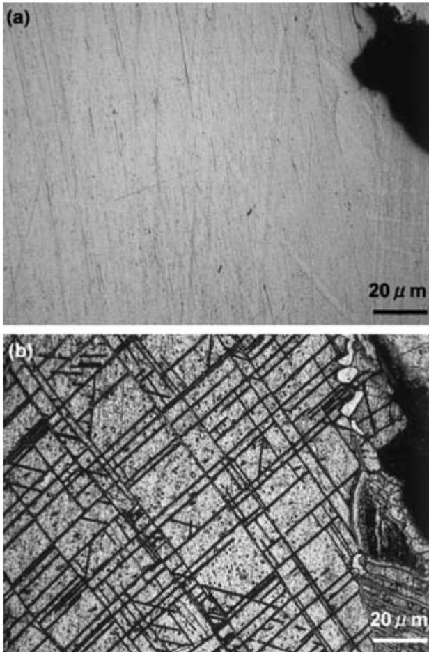
Fig. 4 The kamacite band of Toluca meteorite (a) before etching and (b) after etching, the latter show Neumann lines. Neumann lines are running in several directions through kamacite bands.
