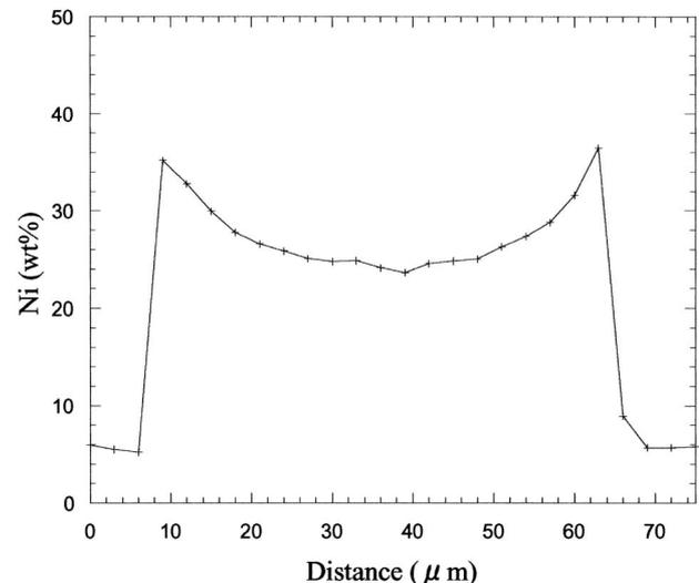
Fig. 6 Ni profile across the kamacite - clear taenite lamellae - kamacite region in the Toluca meteorite.
