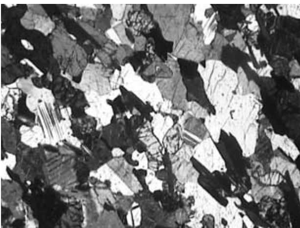
Fig. 4 Photomicrograph showing granulite texture of the two pyroxene granulite wall rock of the Randenigala fault near the Randenigala dam. Long edge of the photograph is 5.2 mm.
