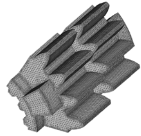
Fig. 3 Finite element model of 1/6 gear.
