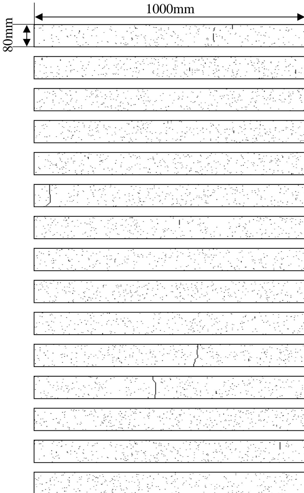
Fig. 6-3 Examples of crack distribution on weld line.
