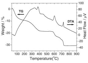
Fig. 2. TG-DTA curves for 0.3 M BT xerogel precursor.
