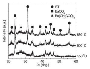
Fig. 3. X-ray diffraction patterns for the BT powders obtained from 0.3 M BT xerogel precursor calcined at different annealing temperature.
