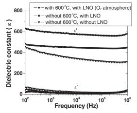
Fig. 5. Dielectric constant and dielectric loss of the BT thin films as a function of frequency.
