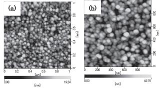
Fig. 7. DFM images of the BT thin films: (a) without  $600^{\circ}$ C preannealing and (b) with  $600^{\circ}$ C pre-annealing.
