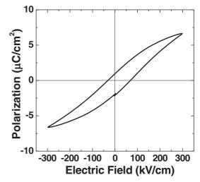
Fig. 6. Hysteresis curves of the BT thin films with the LNO seeding layer and  $600^{\circ}$ C pre-annealing.
