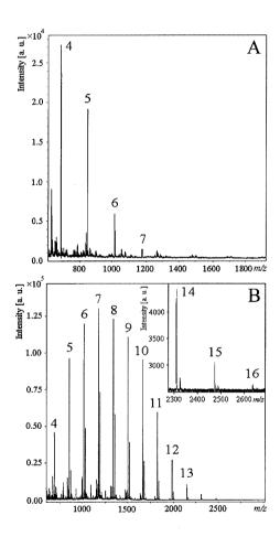
**Figure 1.** An EG I-mediated reaction was carried out using cellobiose or cellotriose as starting material. MALDI-TOF mass spectra of the reaction products are shown: (A) cellooligosaccharides from cellobiose and (B) a cellulose-like substance from cellotriose.
