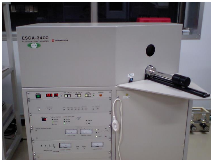
Figure 17. ESCA-3400 device image used for XPS measurements.
