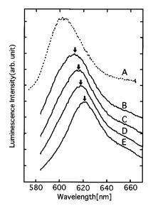
FIG. 1. Luminescence spectra in the reflection experiment from a colloidal solution containing  $1 \times 10^{-3}$  M sulforhodamine 640 in water and polystyrene spheres for different excitation pulse energy. (B) 0.0001 (mJ); (C) 0.001 (mJ); (D) 0.01 (mJ), and (E) 0.1 (mJ). (A) is the luminescence spectrum in a pure dye solution in water of molecular density  $1 \times 10^{-7}$  M. Arrows indicate the luminescence peak.
