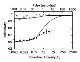
FIG. 4. Reflectivity of the excitation light as a function of the excitation pulse energy for two different dye concentrations,  $(\bullet)$   $1 \times 10^{-3}$  M;  $(\bigcirc)$   $1 \times 10^{-5}$  M. Solid and dashed lines are calculated curves of the reflectivity in the absence and in the presence of stimulated emission, respectively, as a function of the excitation pulse energy.
