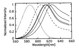
FIG. 5. Solid lines are calculated spectra for excitation pulse energies, 0.0001 (mJ), 0.01 (mJ), 0.1 (mJ), and 1 (mJ) consecutively from left to right for the colloidal solution of the  $1 \times 10^{-3}$  M dye concentration. Dotted and dashed lines are the absorption and the luminescence spectra in the absence of reabsorption, respectively.
