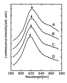
FIG. 3. Luminescence spectra in the transmission experiments from the colloidal solution containing  $1 \times 10^{-3}$  M sulforhodamine 640 in water and polystyrene spheres for the excitation pulse energy. (A) 0.001 (mJ); (B) 0.1 (mJ); (C) 1 (mJ), and (D) 4 (mJ). The sample used is the same as for Fig. 1.
