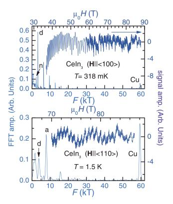
FIG. 2 (color). Examples of dHvA signal measurements on CeIn<sub>3</sub> for two different orientations of **H** together with Fourier transformations. The Cu signal originates from the polycrystal-line Cu comprising the detection coils.
