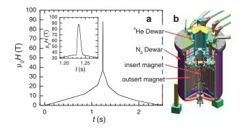
FIG. 1 (color). (a) The H-versus-time T profile of the pulse generated by the combined "outsert" and "insert" magnets. The inset shows the region of the pulse profile provided by the insert magnet in which dHvA measurements in Fig. 2 are made. (b) A schematic of the magnet used for generating the pulse (outer diameter  $\approx 1.4$  m).
