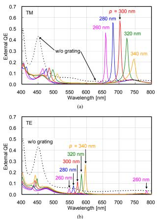
Fig. 4. Calculated spectroscopic external quantum efficiency (QE) for (a) TMand (b) TE- polarized lights. Gate oxide and SOI thicknesses are  $t_{ox} = 100$  nm and  $t_{SOI} = 100$  nm, respectively. Duty ratio of Au L/S grating is fixed at w/p = 0.5.
