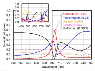
Fig. 3. Spectroscopic response of the optical power components in SOI PD with Au L/S grating. Incident light is TM-polarized. Gate oxide and SOI thicknesses are  $t_{ox} = 100$  nm and  $t_{SOI} = 100$  nm, respectively. Duty ratio of Au L/S grating is fixed at w/p = 0.5. Inserted figure shows spectroscopic responses for wider wavelength range. Transmission is for the power entering the Si substrate.
