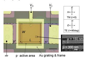
Fig. 2. Top view of the fabricated SOI-MOS p-n photodiode with Au L/S grating. The polarizations with respect to the direction of Au L/S grating are also shown. Au grating is surrounded by a frame to be used as a gate electrode. Dimensions of the p<sup>-</sup> active area are  $L = 50 \mu m$  and  $W = 50 \mu m$ .
