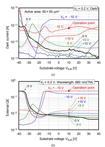
Fig. 8. (a) Measured dark current and (b) external quantum efficiency (QE) as a function of substrate voltage  $V_{SUB}$  for various gate voltages  $V_G$ . Gate oxide and SOI thicknesses of fabricated device are  $t_{ox} = 100$  nm and  $t_{SOI} = 95$  nm, respectively. Grating period is p = 300 nm, and duty ratio is w/p = 0.5. In (b), the wavelength and the polarization of incident light are 680 nm and TM ( $\theta = 0$ ), respectively. The cathode voltage  $V_C$  is fixed at 0.2 V.
