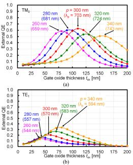
Fig. 6. Calculated peak external quantum efficiencies (QE) as a function of gate oxide thickness with various grating periods p (corresponding to peak wavelengths  $\lambda_p$ ) for (a) TM- and (b) TE-polarized lights. SOI thickness is  $t_{SOI} = 100$  nm. Duty ratio of Au L/S grating is fixed at w/p = 0.5.
