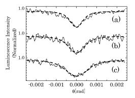
FIG. 1. Solid lines are experimental results for the persistent hole as a function of angular shift  $\theta$  between the writing and reading beams. The sample thickness is L=(a) 1.0, (b) 0.4, and (c) 0.2 mm. The transport mean free path and the absorption length are  $l^*=60 \ \mu m$  and  $l_a=28\ 800 \ \mu m$ , respectively. Dashed lines are theoretical curves calculated on the basis of Eq. (1), where a Gaussian shaped function is convoluted as the experimental angular resolution.
