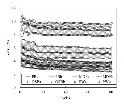
Fig. 5 Ed (GPa) changes during each state over 80 cycles
