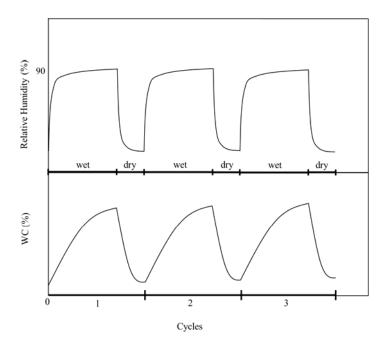
Fig. 1 Schematic diagram of a wet-dry cycle treatment
