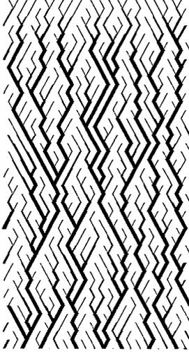
FIG. 1. Typical river-network pattern generated by the Scheidegger river-network model. This run was done on a  $20 \times 40$  square lattice under a periodic lateral boundary condition for an illustration. The width of lines is proportional to the flow rate through each bond where larger flow rates than 8 are indicated by the same width.
