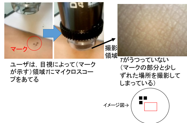
図2 領域 T と異なる場所が撮影される様子 Figure 2 User take different area from area which user wants to take.
