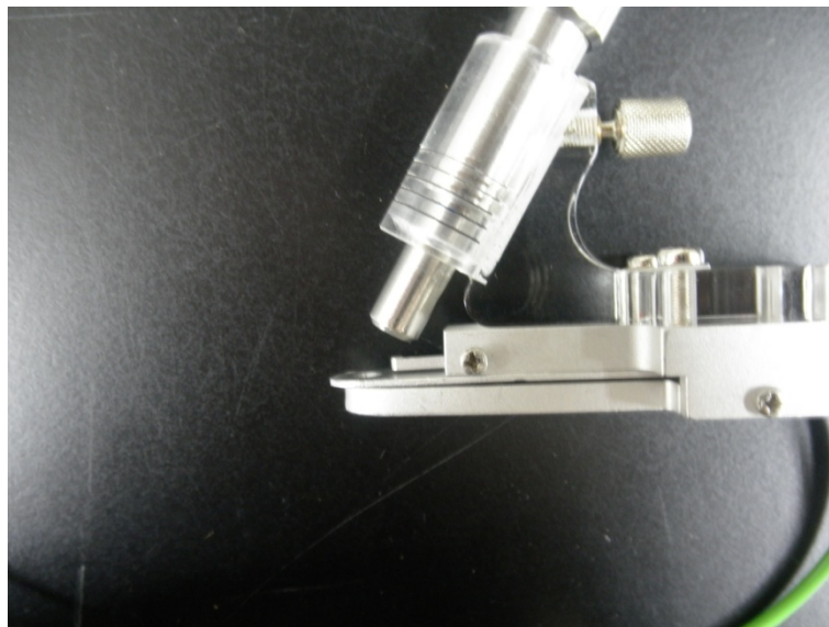
Figure 3. A photo of the leaf clip holder and fiber optics .
