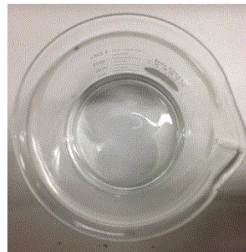
300°C \Rightarrow 99.6% decomp. TOC: 0.59 mg/L
