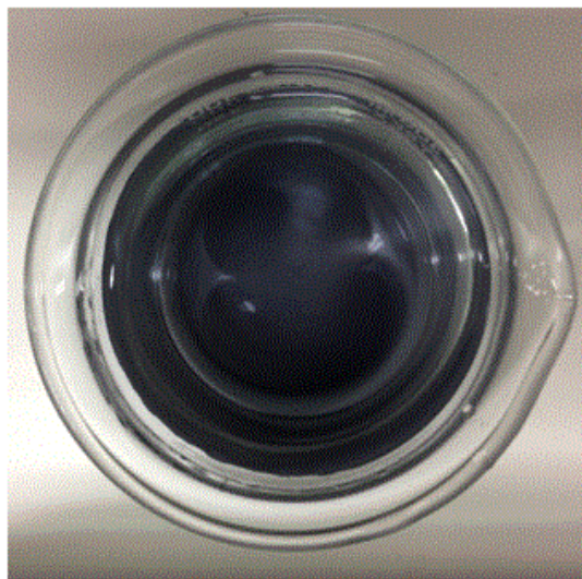
Raw wastewater after biological treatment TOC: 22.0 mg/L
