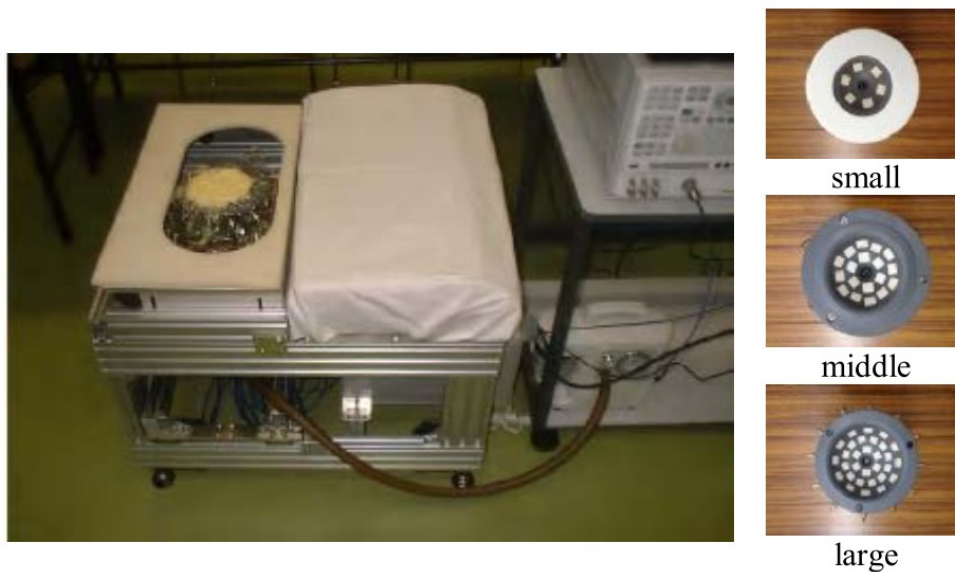
Figure 2.6 Microwave mammography with different sensors [13][14]
